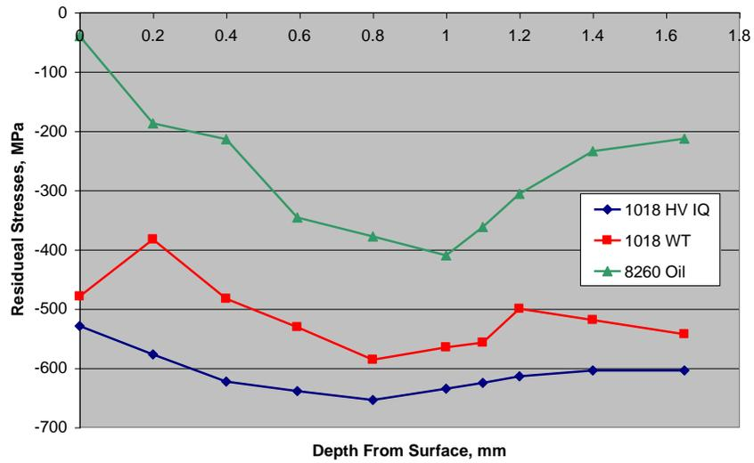
Figure 3 Residual surface stress distribution of carburized 1018 and 8620 Steels
