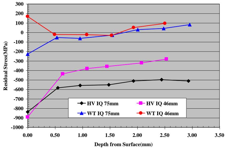
Figure 4 Residual stress distribution for 52100 steels
