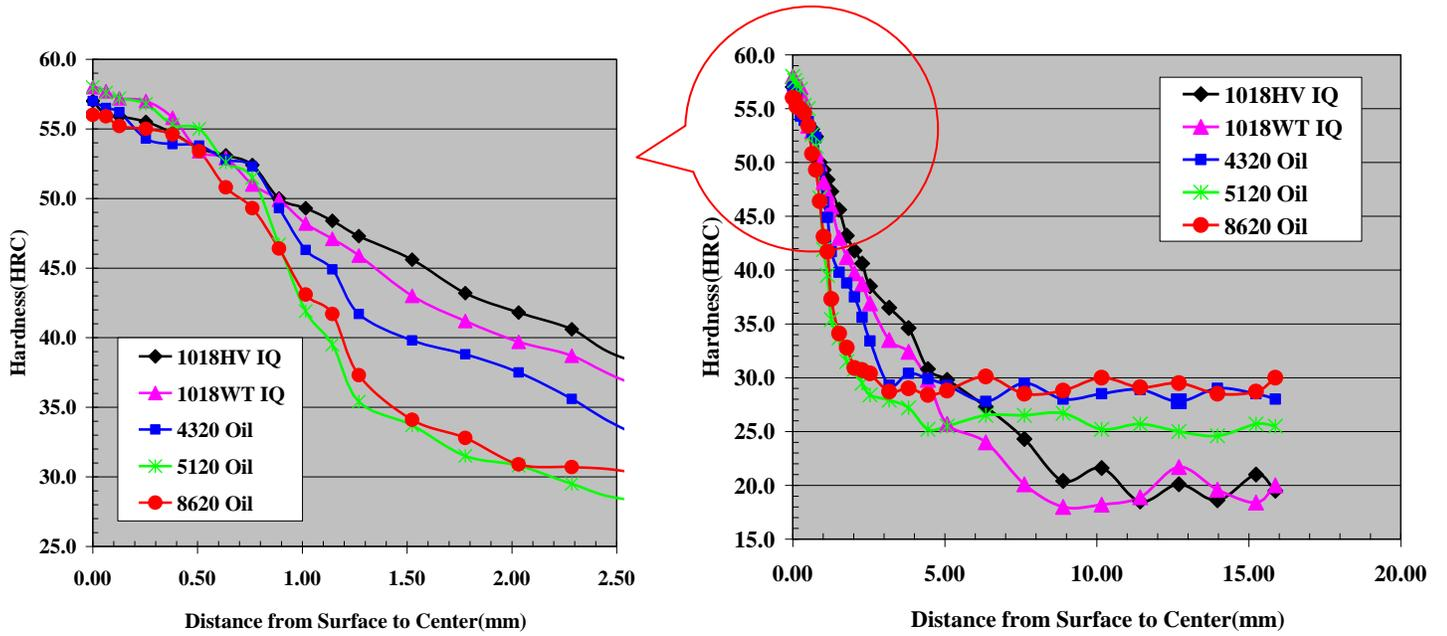
Figure 2 Hardness distribution of carburized 1018, 4320, 5120 and 8620 steels
