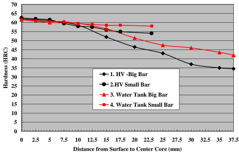
Figure 5 Hardness distribution of 52100 steel
