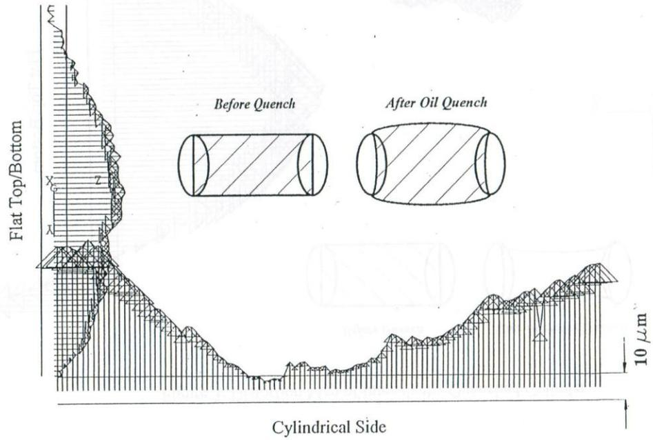
Figure 3: Distortion Map of Intensively Quenched Cylinder
