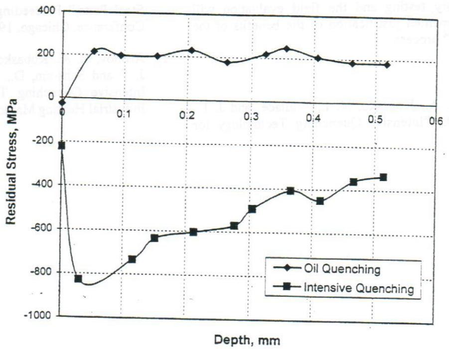
Figure 4 Punch Axial Residual Stresses
