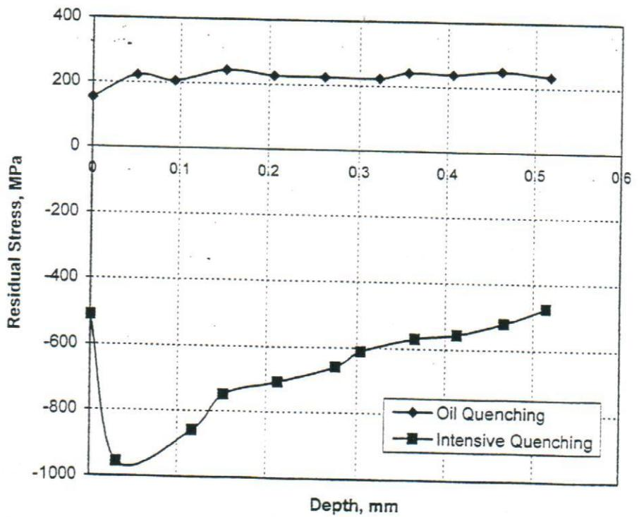
Figure 5 Punch Circumferential Residual Stresses
